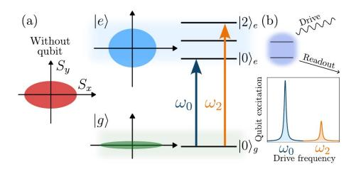
An example demonstrating how a qubit can be used for controlling, detecting, and utilizing the quantum ground state of a ferromagnet is depicted in the figure taken from the article: A. E. Römling, A. Vivas-Viaña, C. Sánchez Muñoz, and A. Kamra. Resolving nonclassical magnon composition of a magnetic ground state via a qubit. <a href="mailto:arXiv:2306.05065">arXiv:2306.05065</a> (to appear in Phys. Rev. Lett.).
